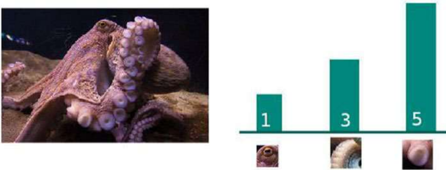
Figure 4-33. Transforming an image into a VBOW vector (Courtesy of Ian London, Image Classification in Python with Visual Bag of Words )
